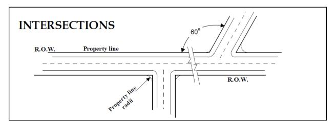
Curb radii at road intersections shall not be less than twenty (20) feet, and where the
