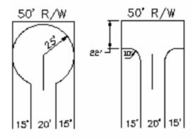
Road width shown as an illustration. Actual width shall be as required by the McMinn Subdivision Regulations based on size and type of road required.
